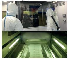
Additive Manufacturing (AM) is a technological revolution in the design and manufacture of components and industrial systems. After a presentation of the process and simulation activities, participants will be led into the laser belt melting additive manufacturing cell to observe the production implementation and discover the safety constraints of metal powder-based processes.
