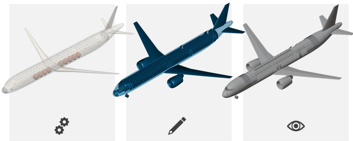
Figure 2: Cabin representations at different development stages, from left to right: conceptual, preliminary and detailed design phase (modified from [12]).
