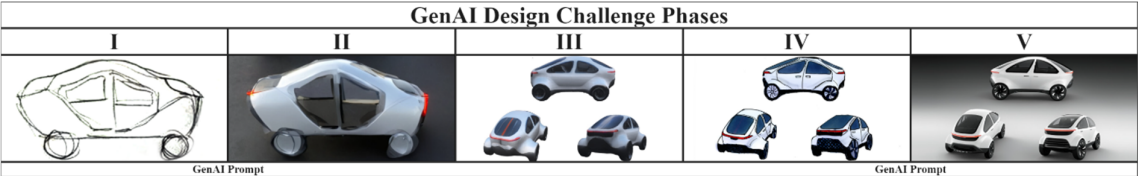
Figure 1. Hand sketch (I), refined sketch using GenAI (II), three-view layout from 3D model (III), freehand sketch on top of three-view layout (IV), finished three-view proposal (V) Participants underwent a one-hour training session on Vizcom which covered its tools and proposed workflows for a three-hour design challenge via teleconference (executed a week later). The task was to design a four-passenger ultra-light autonomous vehicle for smart cities in 2040. The challenge was structured into five phases: 1) 15 minutes for reflection and objective-setting using the Golden Circle methodology [16], where participants outlined a user type, the vehicle’s purpose, and how it met design goals; 2) 20 minutes for freehand-sketching of side views (paper or digital) (Figure 1, Step 1), then for the creation of GenAI iterations and selection of one to pursue; 3) 25 minutes for refinement of the selected idea (Figure 1, Step 2), the creation of a rough GenAI 3D model and a concept page layout with side, front, and rear views (Figure 1, Step 3); 4) 40 minutes for hand-sketching over the concept page to refine the rough 3D; 5) 40 minutes for refinement and creation of the final three-view proposal. Reflection periods (10 minutes each) followed phases 3 and 5, enabling participants to document their approach to creating GenAI images and compare differences, benefits, and downsides of GenAI tools versus traditional methods. A week later, a one-hour post-challenge session between the participants and the researchers was held to reflect on the challenge experience, the role of sketching, the impact of GenAI, and implications for design education. Finally, researchers evaluated and analysed the data.
