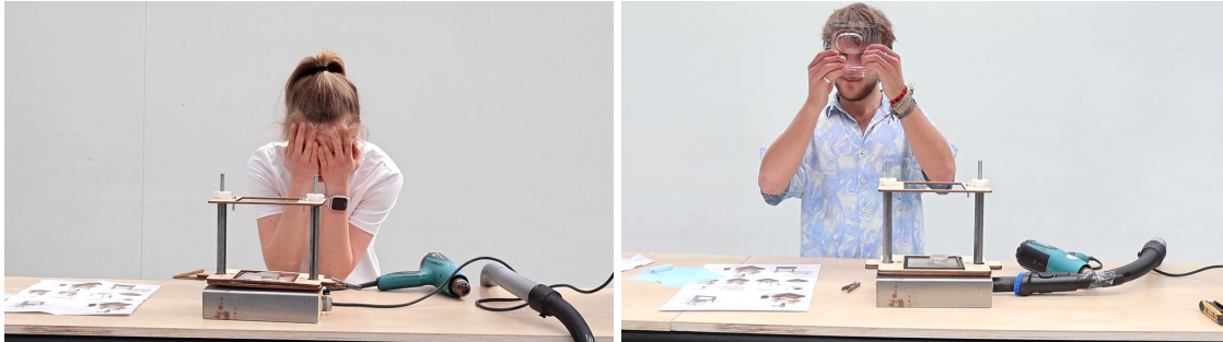
Figure 2. Two students experimenting with the thermoforming machines. Left, the student realises it had to connect the vacuum cleaner's hose to make the process work. Right, a successful realisation of a part using thermoforming
