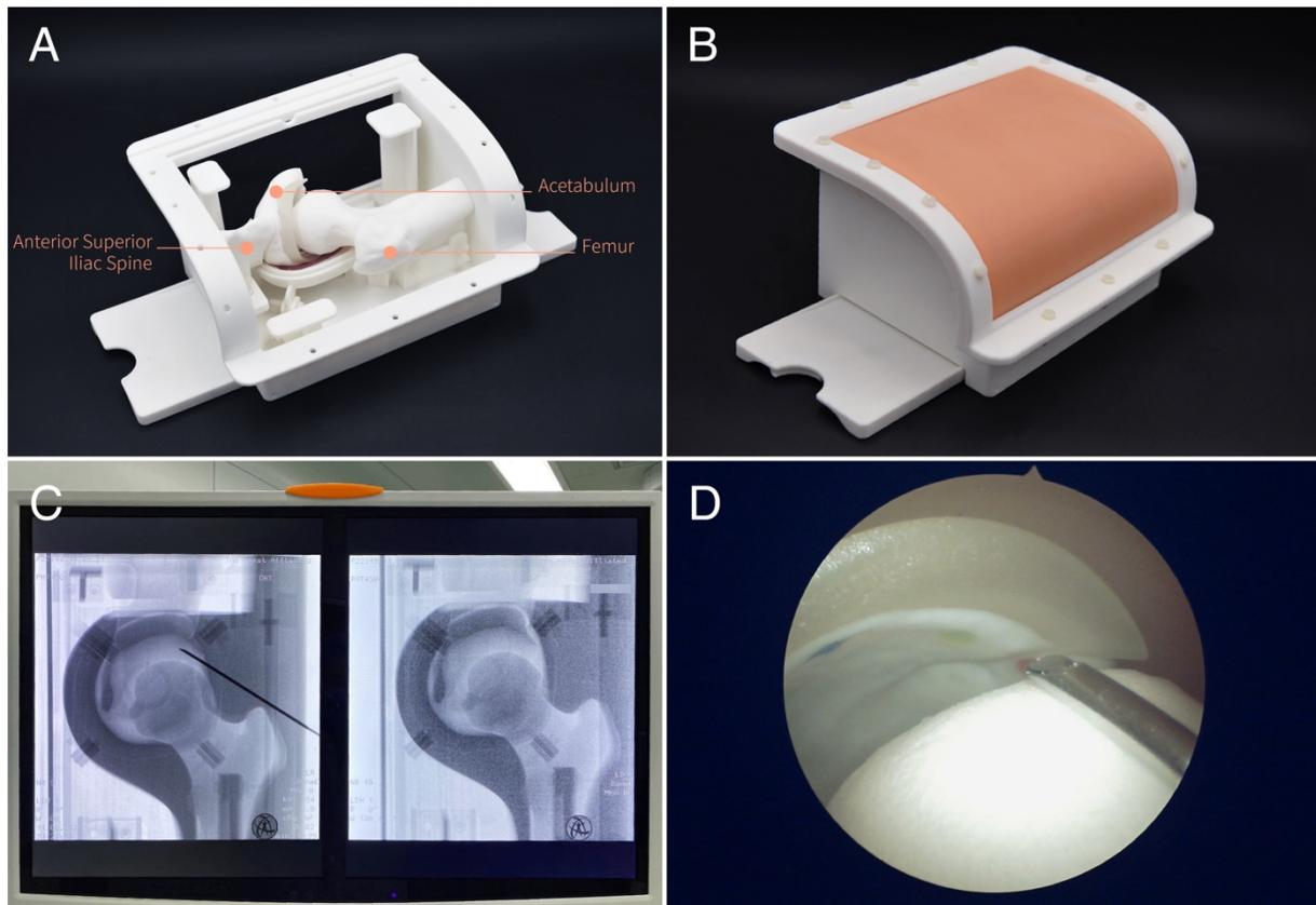
*Figure.2 The 3D printed simulator: (A) The 3D printed bony structures of the simulator; (B) Assembled simulator with the silicon component; (C) Fluoroscopic images for the portal placement process; (D) Arthroscopic view of the process for establishing the distal anterolateral (DALA) portal.*
