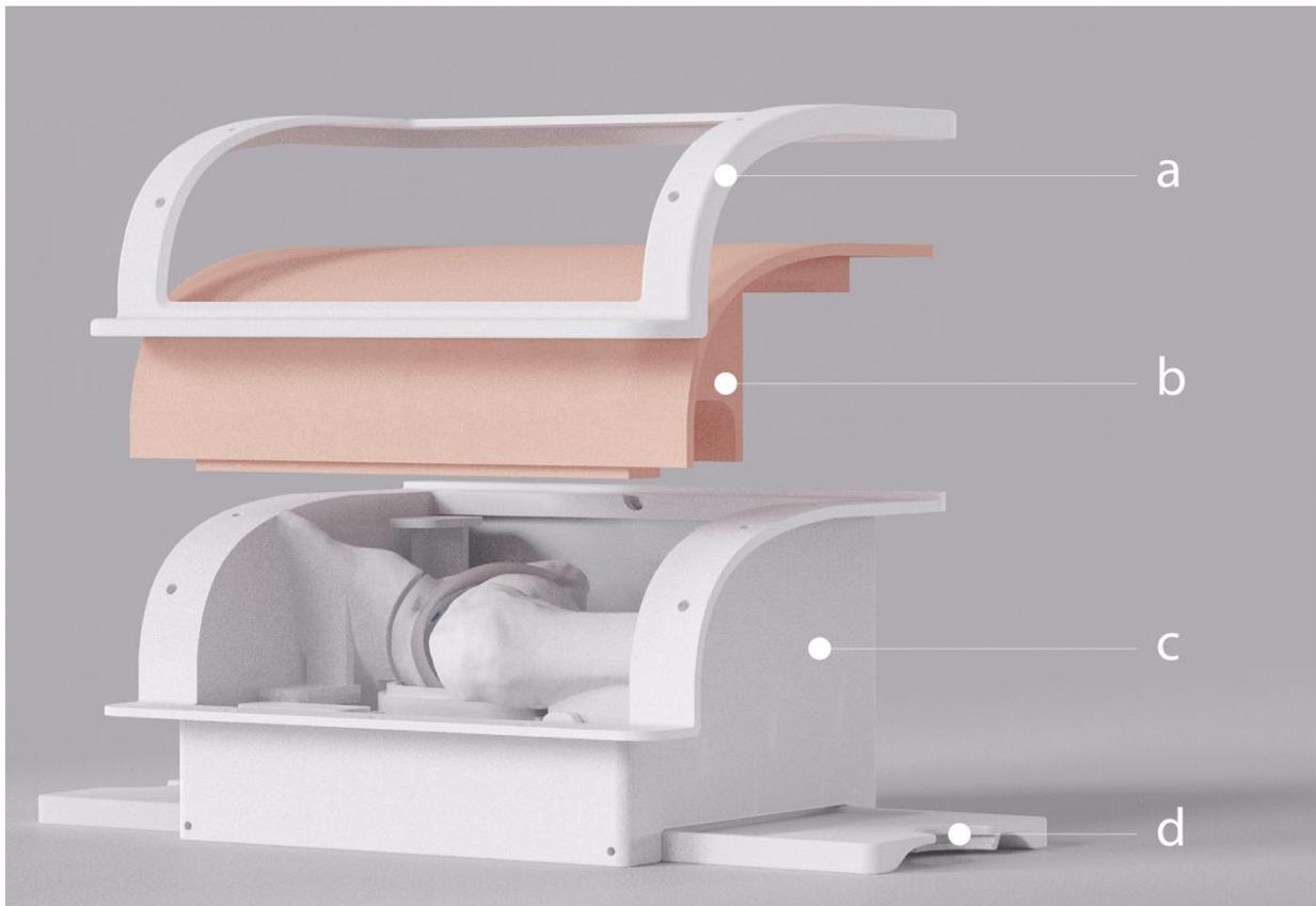
*Figure.1 Main components of the simulator: (a). clip frame to fix the soft component, (b). soft component to simulate the soft tissue, (c). container for holding all the bony and supporting structures, (d). bench fixer used in tandem with a bench vise to secure the simulator onto the table (foldable).*
