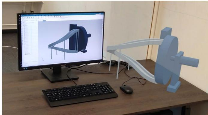
Figure 3 Augmented reality photo showing a mock-up of the hybrid AR computer workstation. An exported triangulation of the CAD model is shown on the HoloLens 2 using the built-in application *3D Viewer*.
