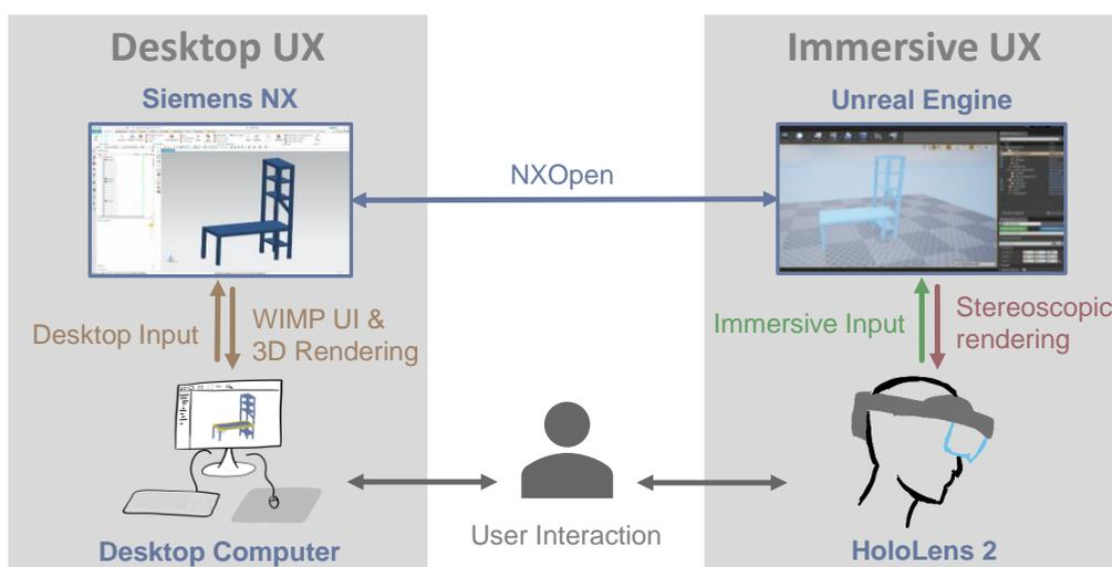
Figure 2 Overview of proposed system components and their interactions
