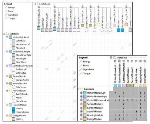
Figure 3. Left: DSM implemented in CSM, Right: Module View with summed interfaces in CSM
