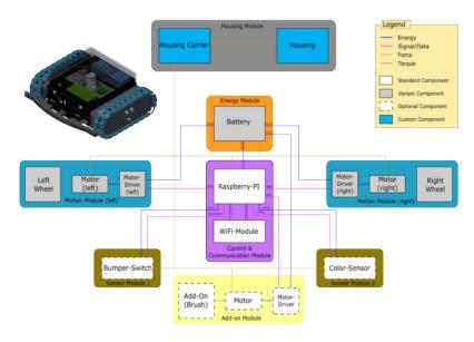
Figure 2. PFIG of the Product Family and CAD-model of the prototype under development These data and data correlations can now be stored in a SysML-Model in CSM. This builds
