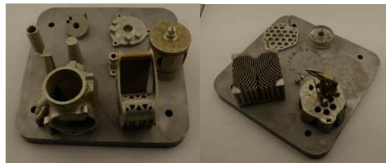
Figure 3. The base plate after the SLM process, before the students removed the parts and post-processed them
