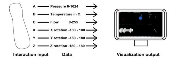
Figure 5. Diagram shows the connections between the TUI and GUI that consist of six different values and their individual ranges. An Arduino captures the data from the various sensors.
