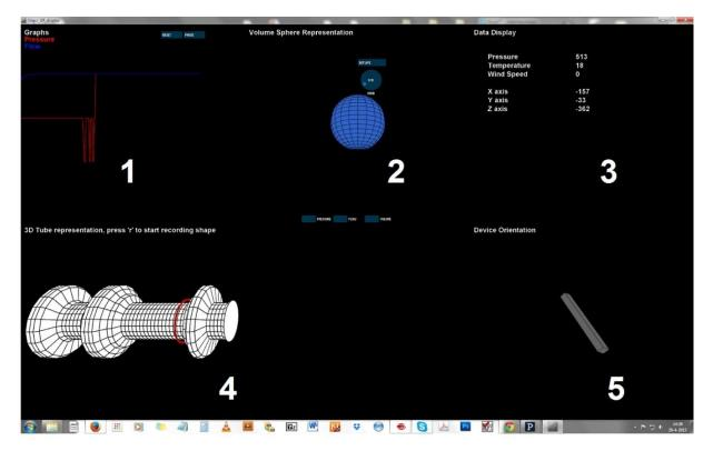
Figure 6. Five data representations; pressure graph display (1), cumulative volume (2), plain text data XYZ (3), generated 3-D shape (4) and rotational orientation and position of TUI (5).
