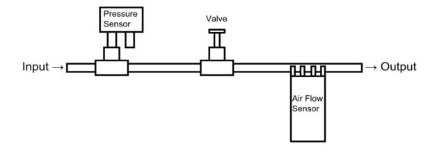
Figure 7. Input and output (IO) of airflow used in the AFIF TUI system.
