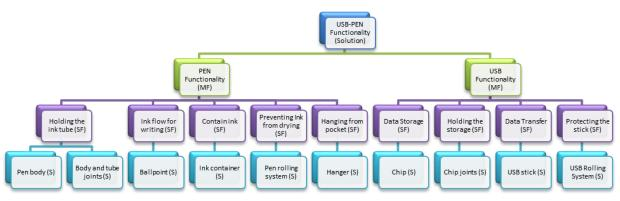
Figure 4. FM Tree of the Designed Structure-Shared Solution (USB + Pen)
