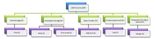
Figure 3. FM Tree of a Typical USB Memory Stick
