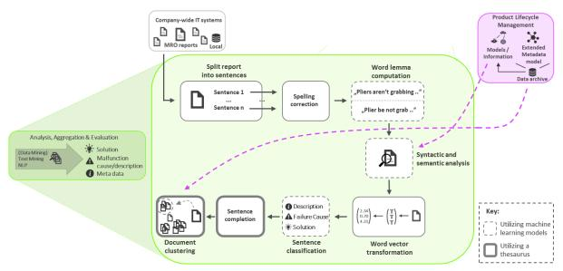
Figure 3. Methodology to process unstructured MRO data
