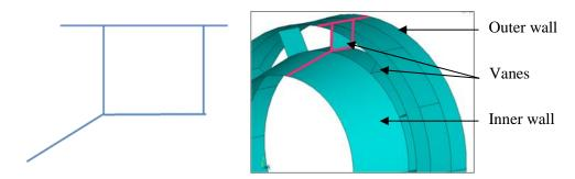
Figure 2. Typical load carrying configuration, highlighted on a static structure
