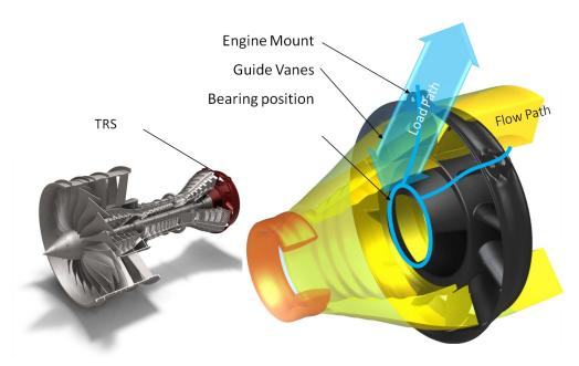
Figure 1. The Turbine Rear Structure (TRS), the flow path (gas) and load path (mechanical)
