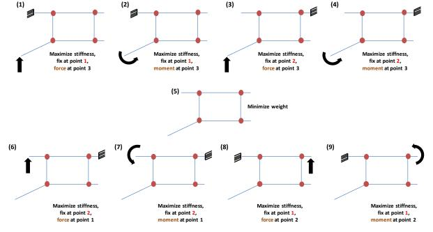
Figure 4. The different loading scenarios on the LCC
