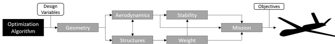
Figure 3. An example of the typical disciplines in MDO frameworks for conceptual UAV design according to the work of Amadori et al. (2006) as well as Jeon et al. (2007)
