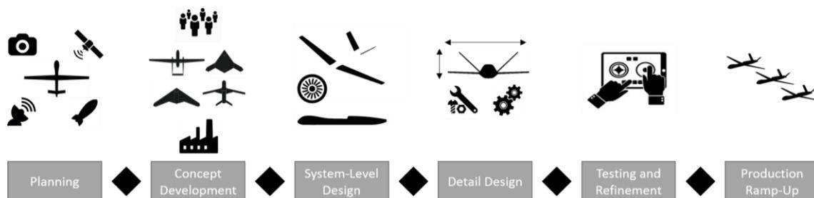
Figure 1. An example of a PDP for UAV design, adapted from Ulrich and Eppinger (2012)
