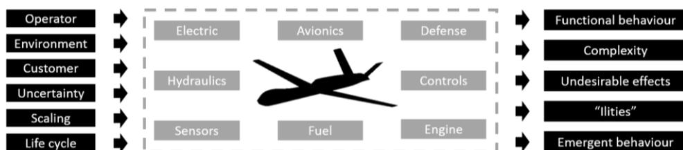
Figure 6. A MDO system engineering approach for UAV design
