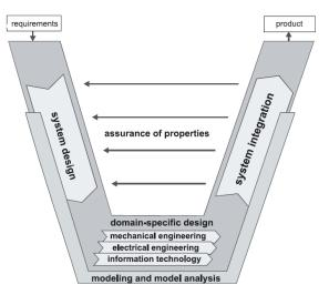
Figure 5. The V-Model according to guideline VDI 2206 (VDI, 2004; Gausemeier and Moehringer, 2003)
