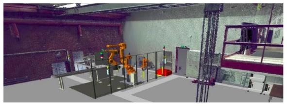
Figure 3. An example of 3D-models in a point cloud environment within a digital factory
