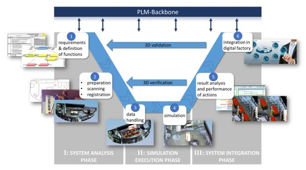
Figure 6. Modified V-Model for Manufacturing (Salehi, 2016)
