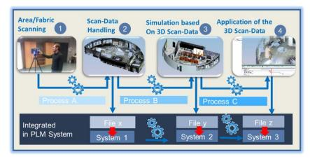
Figure 9. Organized and consistent scanning process with related PLM Backbone
