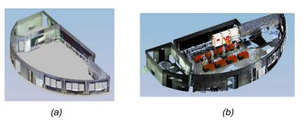
Figure 8. (a): integrated ground plane; (b): CAD generated assembly stations in the point cloud environment
