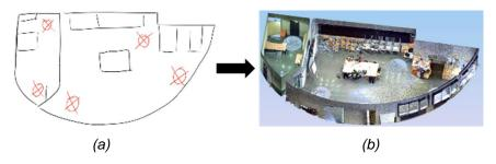
Figure 7. (a): two-dimensional layout draft of scan positions, (b): related point cloud data
