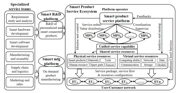
Figure 1. The proposed framework of Smart Product Service System
