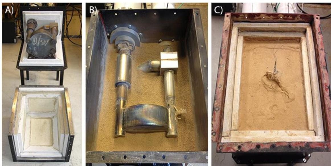
Figure 5. Test setup for: a) Box-type insulation, b) Granular insulation, c) Hybrid insulation. Granular material is Promat Freeflow<sup>®</sup> 220 and panel is Promalight 1000X.
