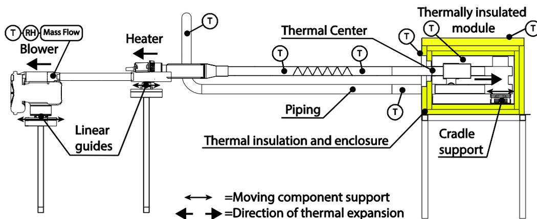
**Figure 4. Example of using Thermal Center at the border between hot piping and components and cool outer enclosure of the insulated box. Here single thermal bridge acts as a structural non-moving support and as a hermetical seal between inner and outer space of thermally insulated enclosure. Instrumentation shown to present experimental setup. Thermal insulation of piping excluded for clarity.**
