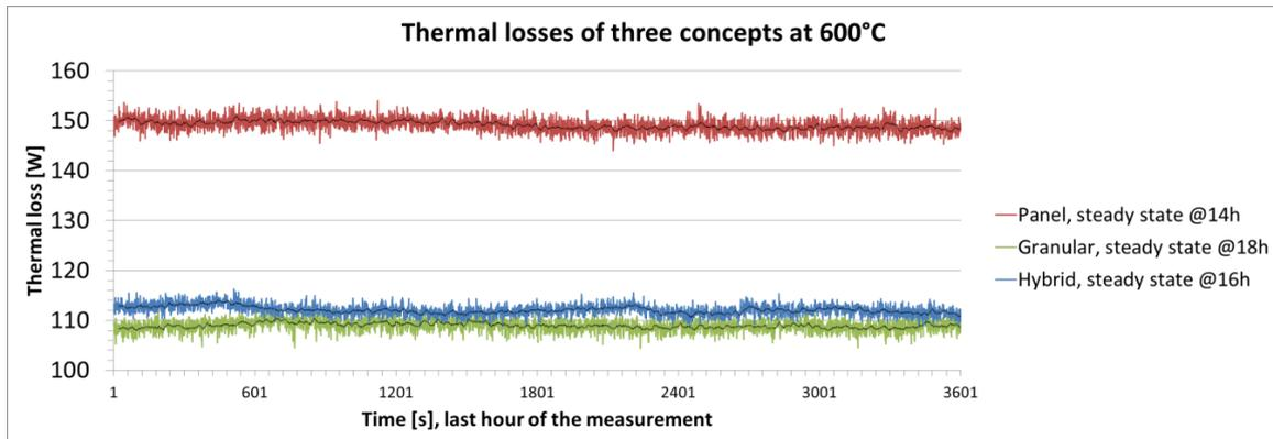
**Figure 6. Thermal losses of three concepts in steady state at 600 °C.**
