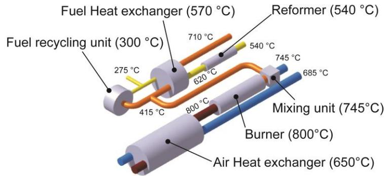
**Figure 3. BoP-module components and their operating temperatures. Instrumentation, valves and actuators excluded for clarity.**
