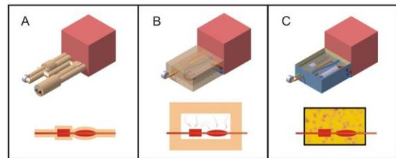
**Figure 1. Insulation concepts A) Individual, B) Box-type, C) Granular insulation.**
