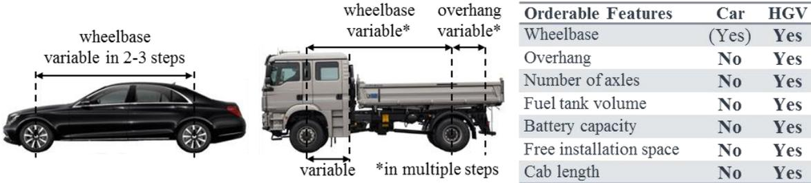
Figure 1. Differences between car and truck
