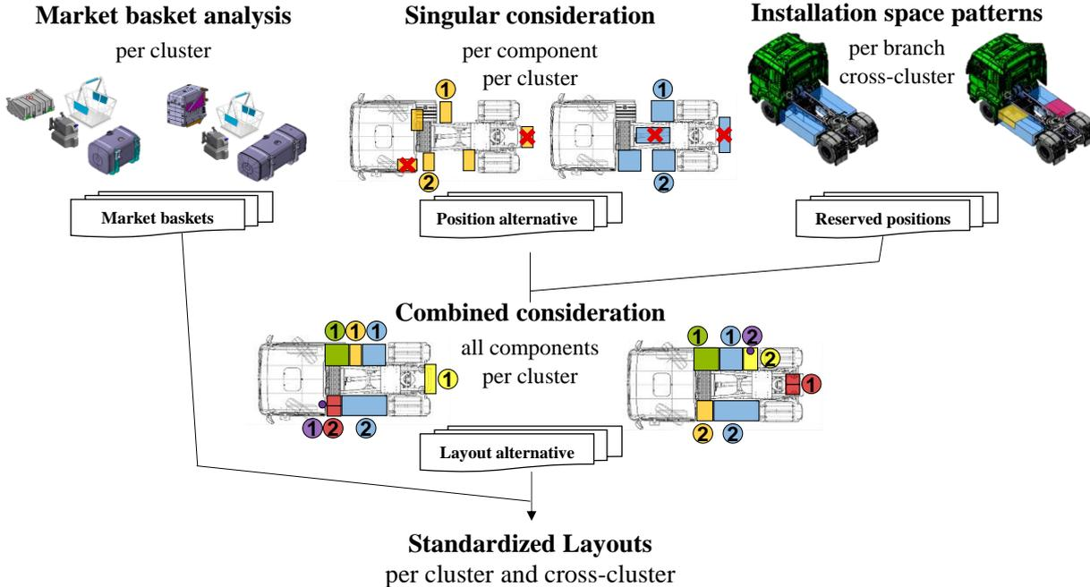
**Figure 3. Methodology for deriving standardized layouts**
