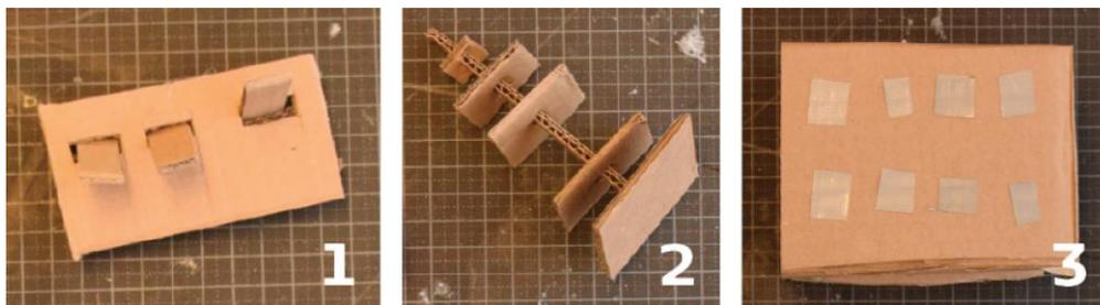
Figure 4 Three prototypes built in the indicated chronological order. No. 1: A 3D puzzle alarm clock. No. 2: A 3D alarm clock puzzle where the pieces have to be put in size order. No 3: A 3D alarm clock with lighted buttons, which the user has to press in a certain order.
