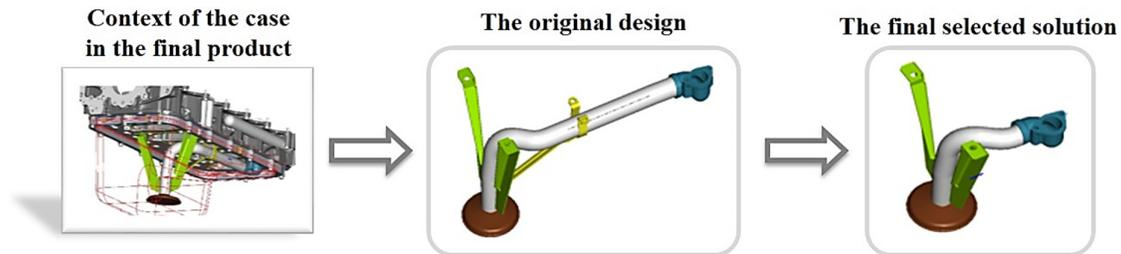
Figure 2. Context of the redesign process of an Oil-Pipe case
