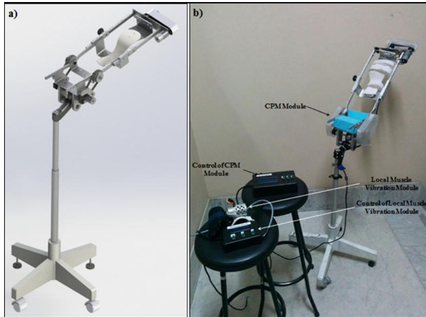
**Figure 5. (a) Isometric view of the selected conceptual design; (b) Prototype of the innovative equipment to rehabilitate elbow and forearm (parts are identified in the figure)**
