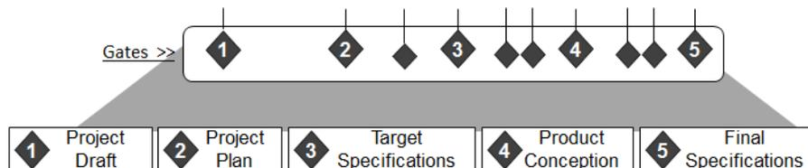
**Figure 3. Gates of the Referential Model for Management and Development of Products.**
