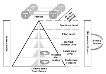
Figure 1. Size range development process, according to Pahl and Beitz, displayed in a product concretisation pyramid (extended and partly adapted from [Sauer 2006])
