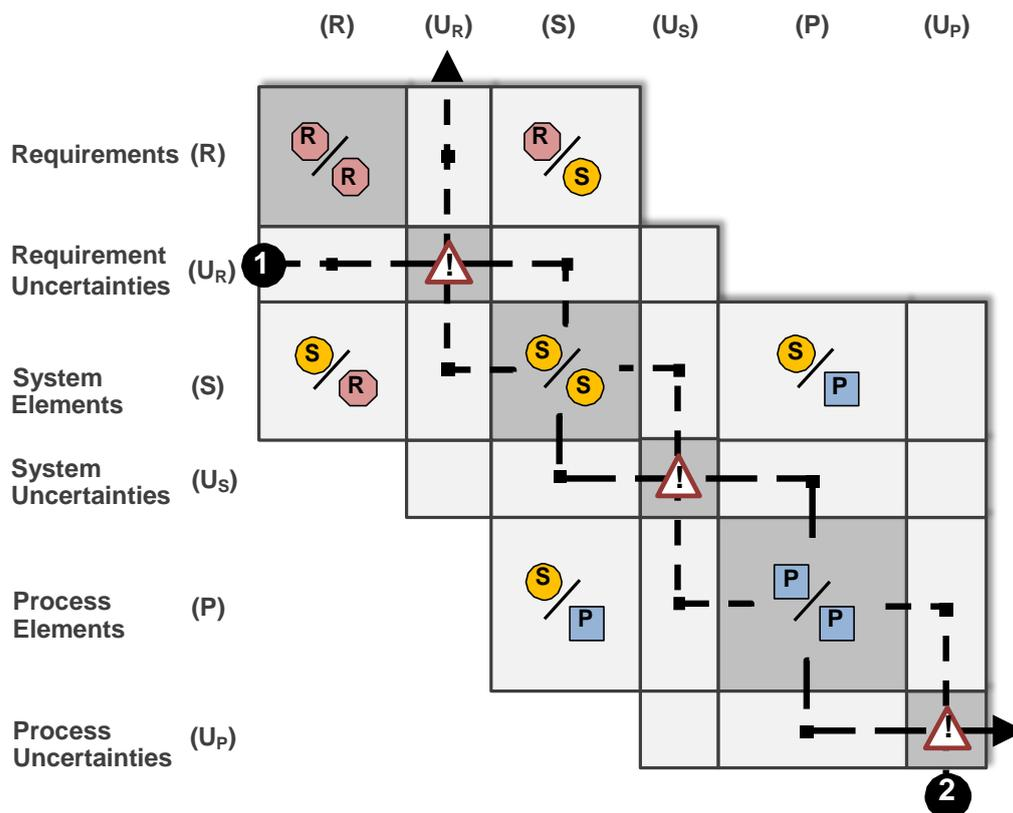
Figure 1: Uncertainty modelling using Multiple Domain Matrices
