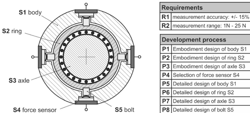
Figure 4: Development of a Radial-Force Measurement unit for rotating axles
