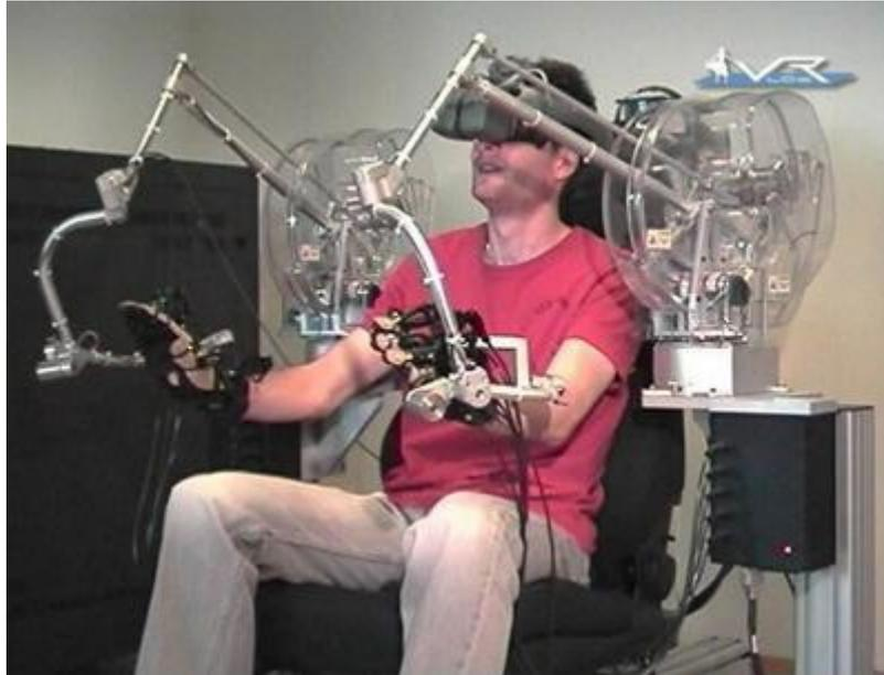
Figure 1 Haptic Workstation of Cyberglove Systems [8]
