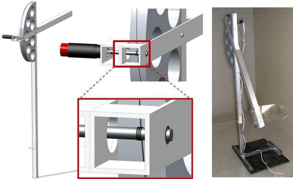
Figure 3 The haptic device as a digital and physical prototype
