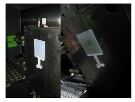
Figure 3. Injection moulding of an RFID tag in a test specimen.
