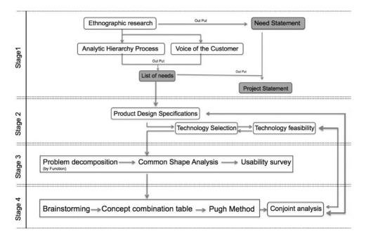
Figure 1. Flow diagram of the PDD process implemented
