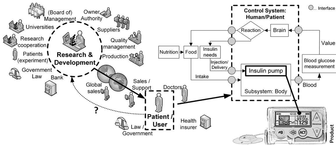
Figure 4. Insulin pump, stakeholders and control loop in a holistic system overview
