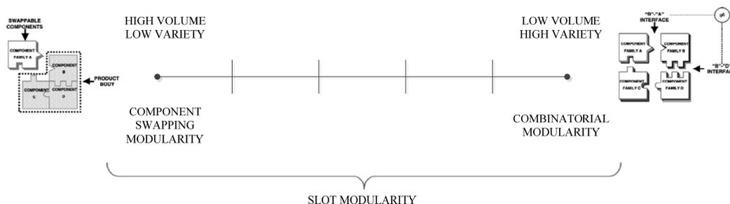
Figure 2. Component swapping - combinatorial modularity spectrum (Salvador et al. 2002).
