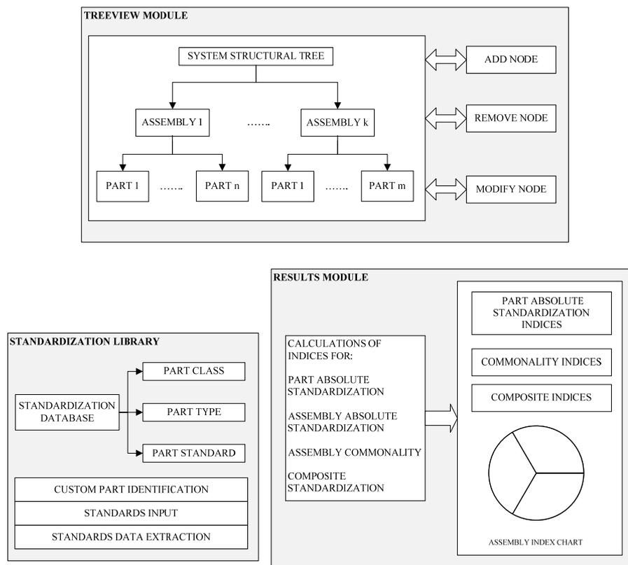
Figure 2. Software main modules and functions
