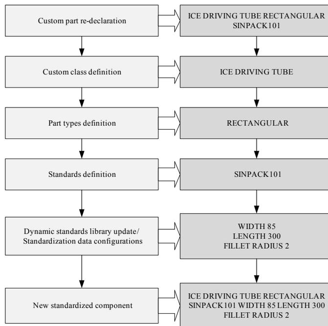
Figure 4. Classification scheme and custom part standardization methodology -Indicative example of the methodology
