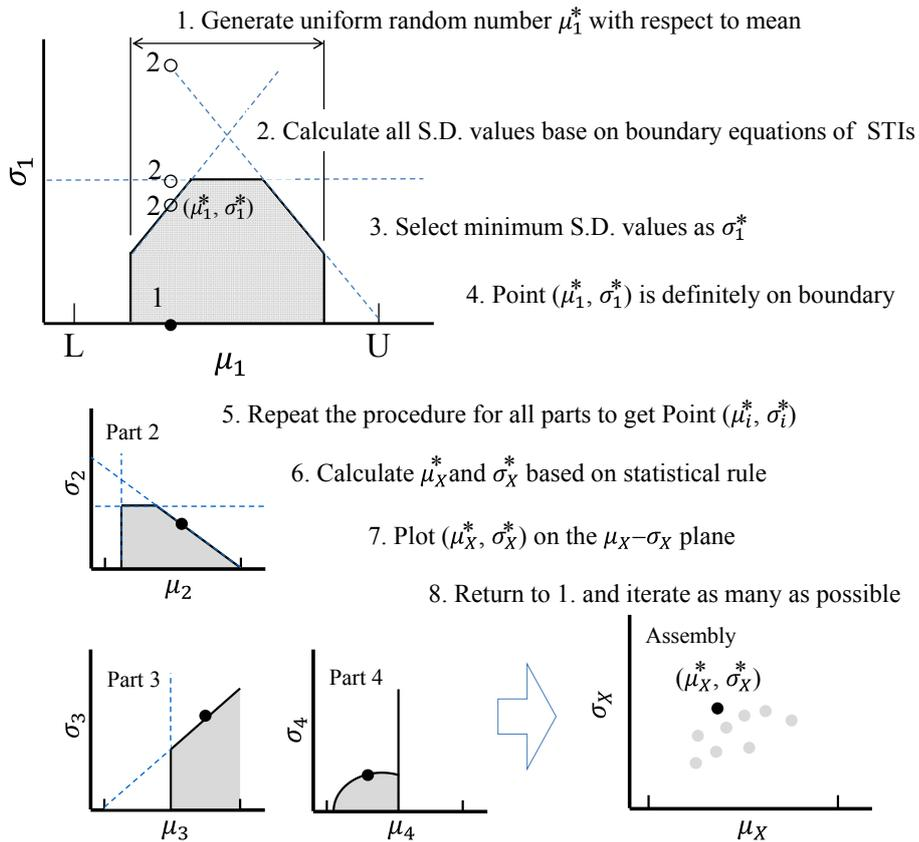
Figure 4. Flowchart of analysis method using Monte Carlo simulation
