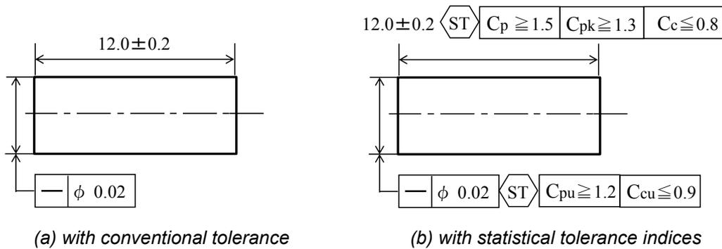
Figure 1. Examples of mechanical design drawing
