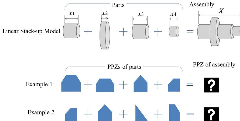
Figure 3. Illustrations of assembly model and Stack-up problem
