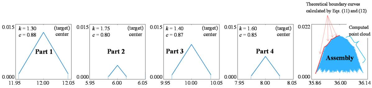
Figure 5. Comparison of theoretical solution and computed solution (Solid curves are theoretical boundary written by equation (9) )
