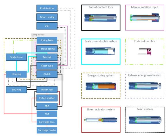
Figure 2. Interface diagram for integrated products – FlexTouch®
