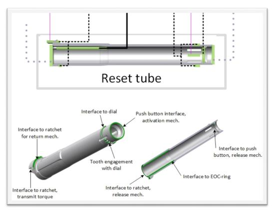
Figure 3. Linking the functional surfaces to the functional overview
