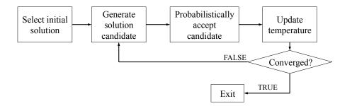
Figure 1. Generalized flowchart for conventional SA.
