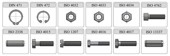
Figure 6. Different standard components for the application of the part recognition concept
