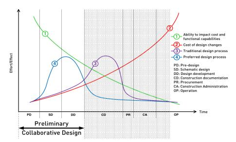
Figure 1. MacLeamy curve. A project that places significant efforts in preliminary design improve its cost-efficiency ratio.
