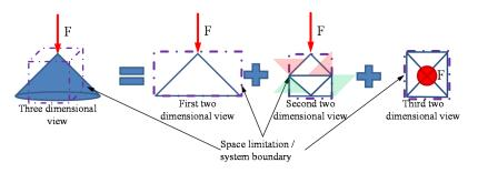
Figure 4. Force Cone and derived structure under consideration of space limitation
