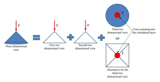
Figure 3. Force Cone and alternative derived structure
