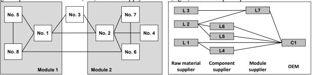
Figure 1. Product architecture and supply network of the ballpoint pen
