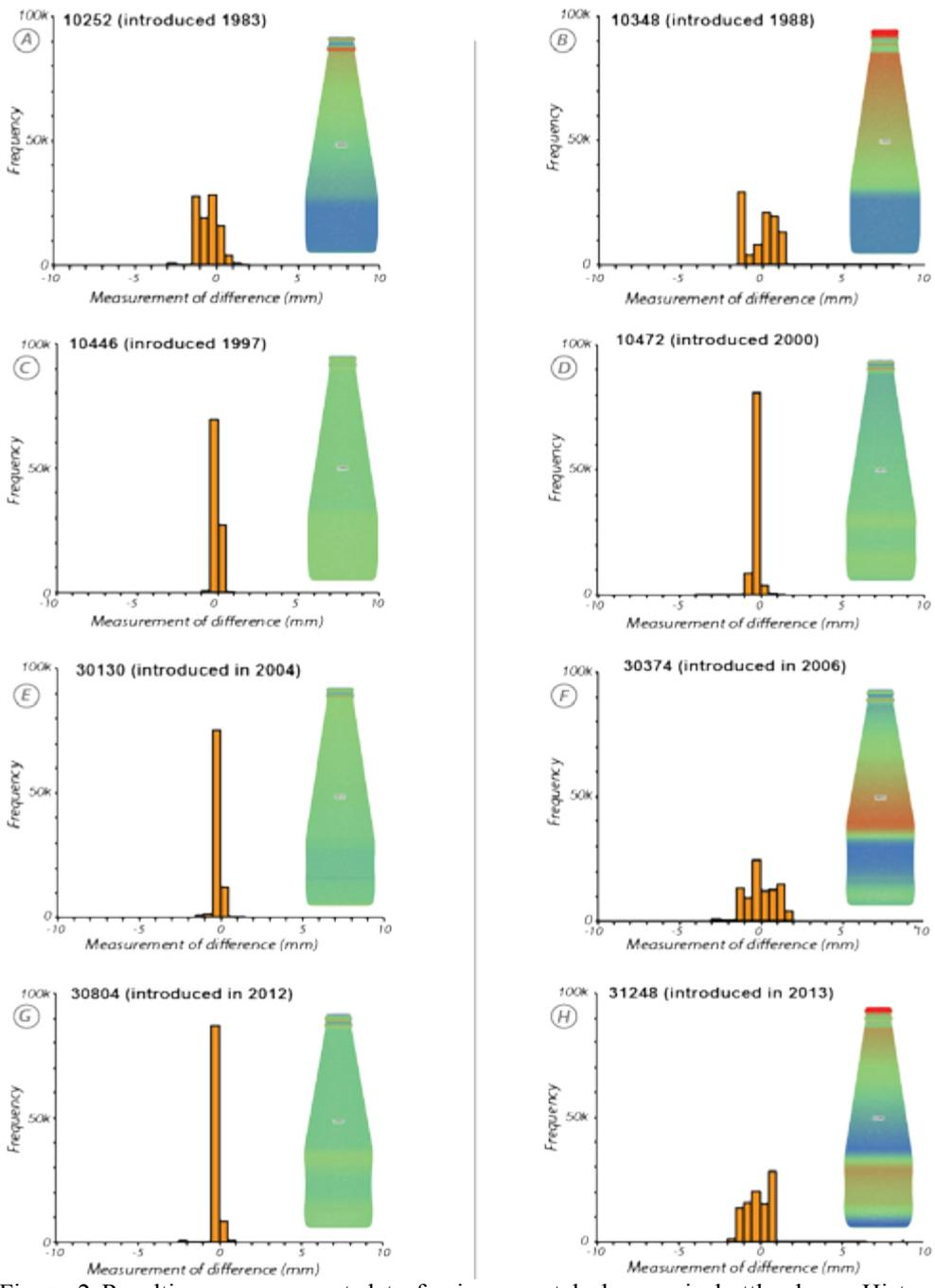
Figure 2 Resulting measurement data for incremental changes in bottle shape. Histograms show the distribution of degree of difference of surface comparison. Data is also visualised on the bottle surface using a colour ramp that accompanies each plot.
