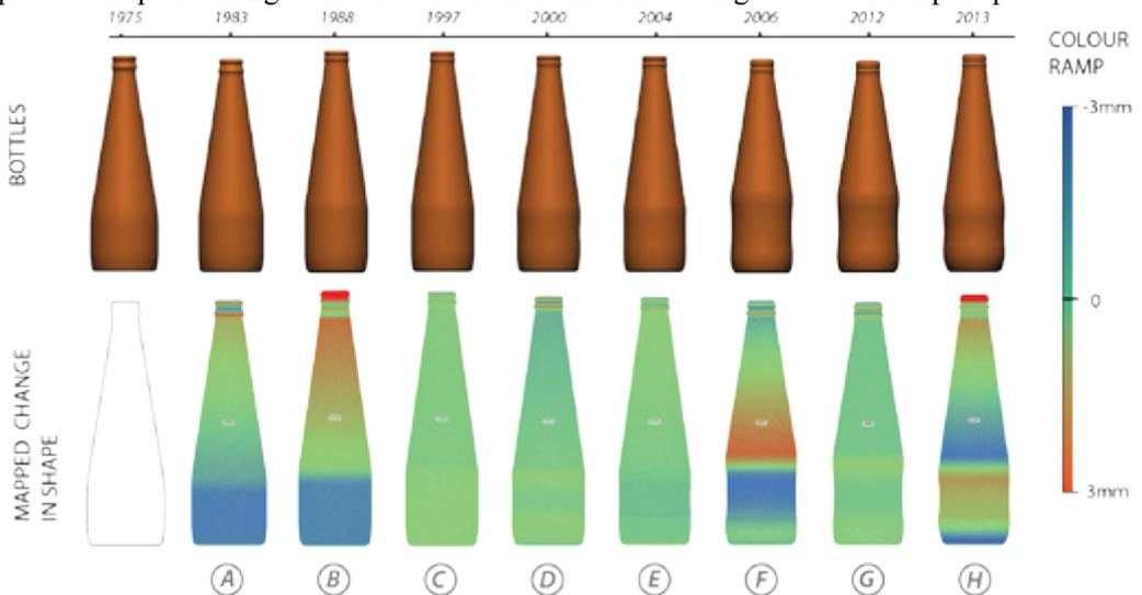
Figure 1. Evolution of bottle designs. Note change in shape mapped using the colour ramp (right) on each successive bottle design.
