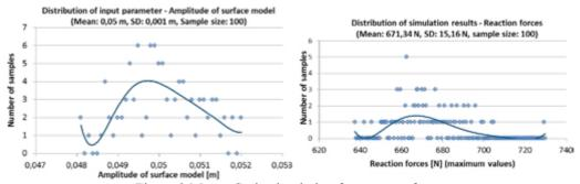
Figure 3 Monte Carlo simulation for actuator force
