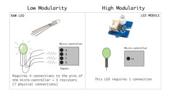
Figure 1. Comparing the modularity of two LED components.
