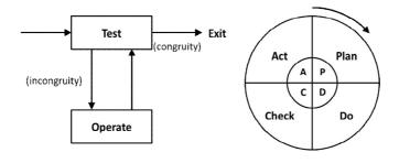
Figure 10.1. Basic models of iteration: TOTE unit (left) and PDCA cycle (right)
