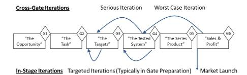
Figure 10.5. In-stage and cross-gate iterations
