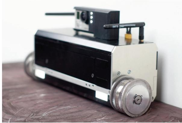
Figure 1. Final prototype of the exemplary project Ship Inspection Robot
