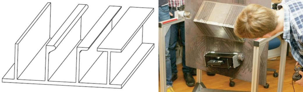
Figure 2. Defined profiles for the robot to climb (left) and the turnable test rig, with which all relevant obstacle features can be simulated with variable direction of gravity (right)
