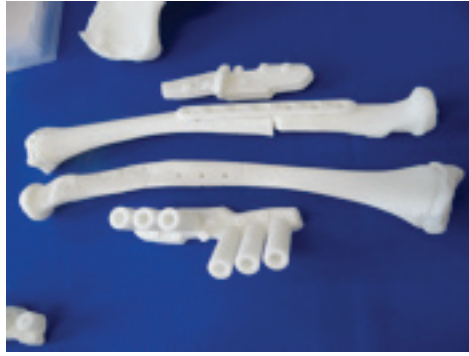
Figure 1. Surgical guides are developed using 3D printed practice bones and 3D printed (photo c J.Loy)
