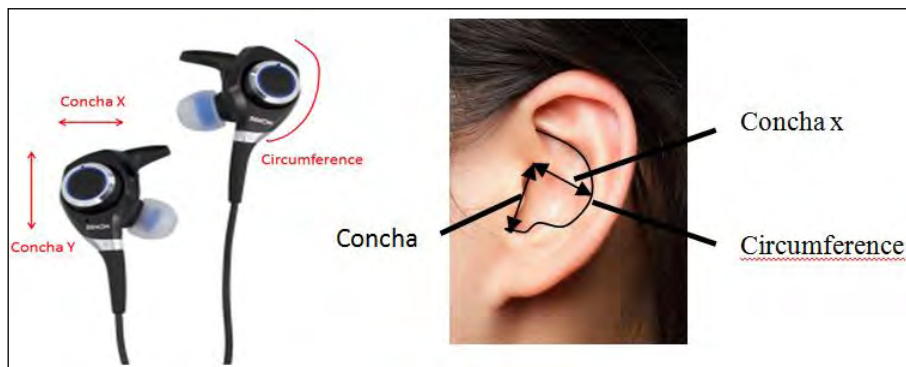
Figure 1. An image of the prototype and respective the critical ear dimensions
