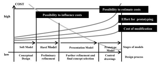
Figure 6. The possibilities costs of model making in relation of design process, adapted from Ehrlenspiel et al. [2007]
