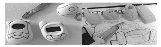
Figure 1. Sample of soft model (source from Industrial Design UiTM, Malaysia)
