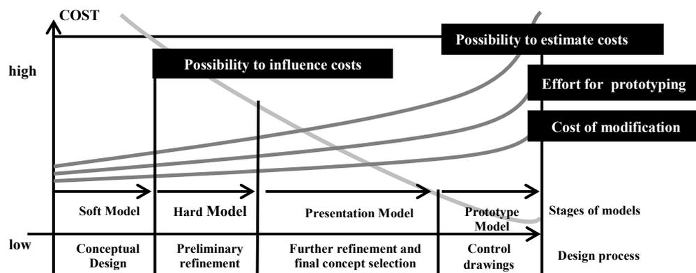
Figure 6. The possibilities costs of model making in relation of design process, adapted from Ehrlenspiel et al. [2007]
