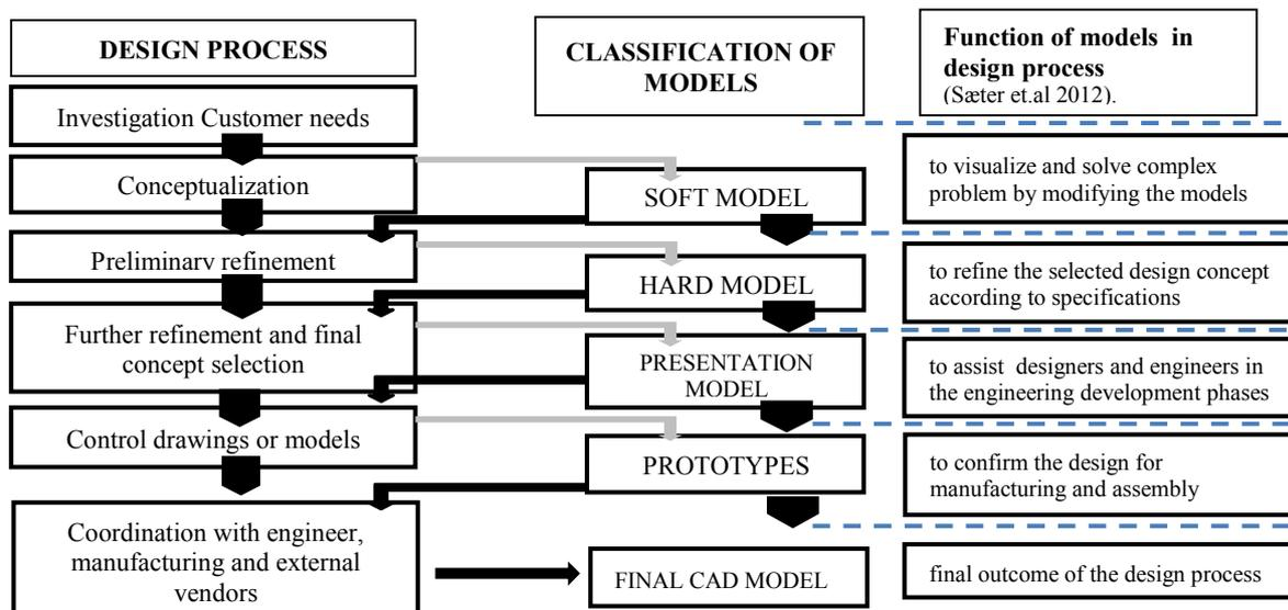
**Figure 5. The linkage of models and prototypes with the different stages of the design process according to multiple researchers (adapted from [Ulrich and Eppinger 2012])**
