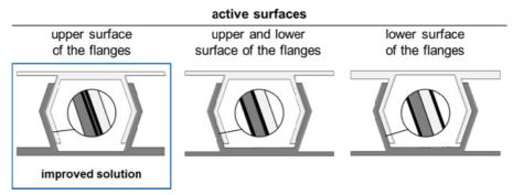
Figure 12. Using returned cognition in designing a snap connection
