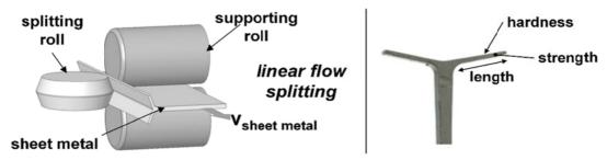
Figure 1. Linear flow splitting - process and product
