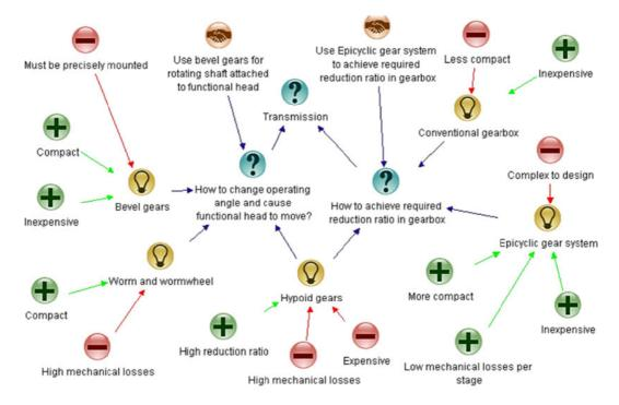
Figure 5. An example of gear transmission considerations and idea evaluation
