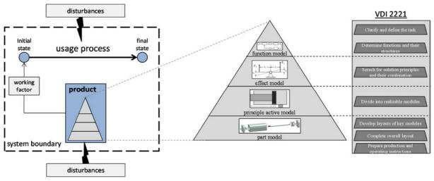
Figure 4. Systematization of level of information [Heidemann 2001], [VDI 2221]
