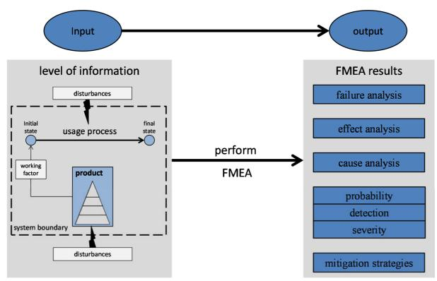
Figure 6. Input and output of an FMEA
