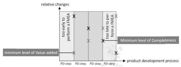
Figure 13. Determination of the ideal time to perform an FMEA
