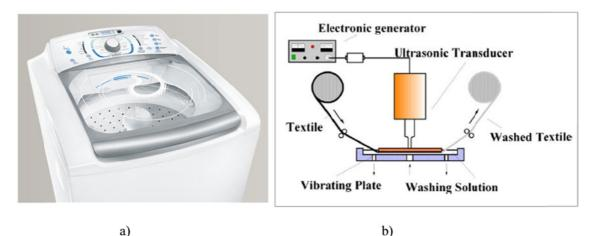
Figure 2. a) Electrolux Ultra Clean washing machine ['Electrolux annual report 2011' 2013],b) Scheme of the ultrasonic system for textile washing [Gallergo-Juarez et al. 2010]
