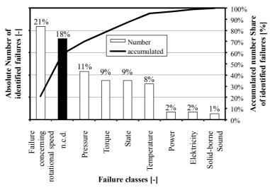
Figure 1. Failure classes and Pareto analysis, see [Schenk 2012]
