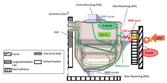
Figure 4. Pole Side Impact on a structural concept of a HVS (C&C<sup>2</sup>-M)
