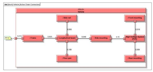
Figure 6. Internal block diagram: Energy transfer of the load path (pole side impact) in a block definition diagram (proportional values added for comprehension) based on a vehicle crash simulation
