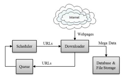
Figure 2. The high level architecture of a standard web crawler (see Castillo 2004)
